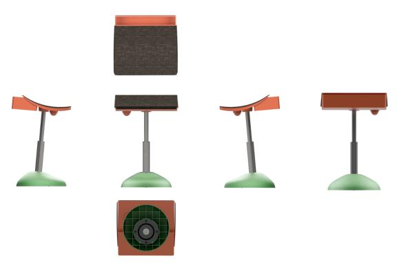
Figure 11 – Proposed Design Third Angle Six-View Projection
