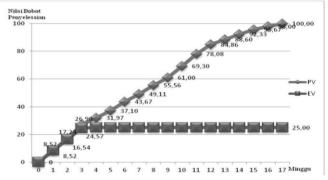
Fig. 1 S Curve Feeder STO Garut Modernization Project
